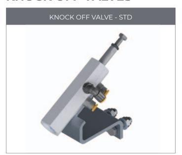
Knock off valve STD is mounted on the cylinder cradle, it is delivered with a special bracket to allow easy installation and precise setting of this limiter. It is pneumatically operated, the mechanical adjustment allows it to be used with full range of Hyva front cylinders. Usage of this valve assures precise operation and smooth limitation of the stroke which results in significant increase of the cylinder and hydraulic lit lifetime.
