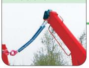
Walk on protection guards, for protection of the piston rod.
