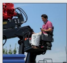
Top seat with servohydraulic controls
