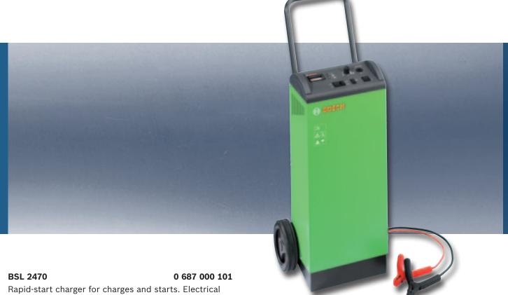
Rapid-start charger for charges and starts. Electrical components are protected against damage during starts and charges (DIN 40839, interference emission level I). Voltage selection switch for 12 V and 24 V. Continuously adjustable charge current. Switch for exhaustive-discharge batteries. Switch for temperature-compensated charges. Charges based on WU charging characteristic. Ampere meter, charging cable 3 m, with fully insulated charging clamps, overcharge protection.
